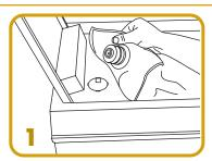
Place the nozzle of the bag with cap installed tightly inside the opening of the splash guard located inside the bag chamber
